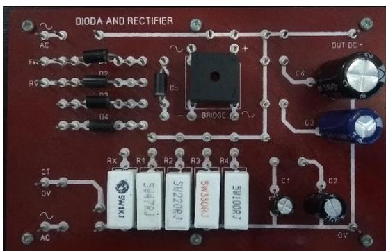
Gambar 2. Modul *Dioda and Rectifier*
